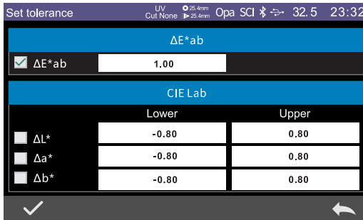
Figure 30 Interface of System Tolerance Settings
