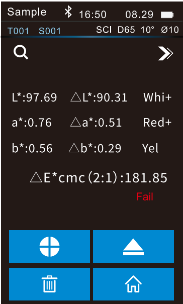
Figure 34 Calculation of Color Difference Using \Delta E CMC (2: 1)
